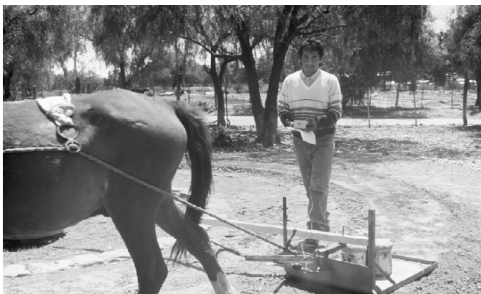
Figure 2: The test track for single equines pulling a variable load with different harnessing arrangements
